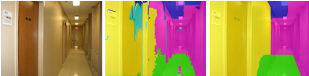
Figure 5. Failure case for the five regions layout. Since the dataterm ( center ) is very misleading, the ordering constraints do not allow to recover the desired solution. From left to right : input image, dataterm, result with ordering constraints.
