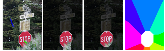
Figure 11. Beyond existing approaches, the proposed framework allows to model priors on convex shapes. From left to right : input image with user scribbles, Potts partitioning, partitioning using the convex shape prior, prior encoding. The prior is modeled by a n -gon, here an octagon, with edges pointing in all directions.
