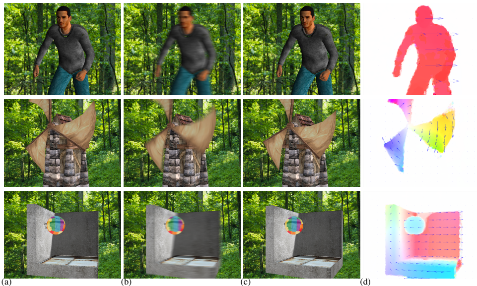
Figure 5: Scenes Ben , windmill and corner : Input images I_1 , I_B and I_2 (a)-(c), motion field calculated with our method (d).
