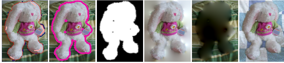
Figure 3: Segmentation of the Rabbit image taken from [12]. From left to right: Original image with constraints and binary segmentation border overlaid in red. Automatic determination of matting regions. The resulting \alpha -map. The image I_F and I_B . A composition of the extracted image with a new background.
