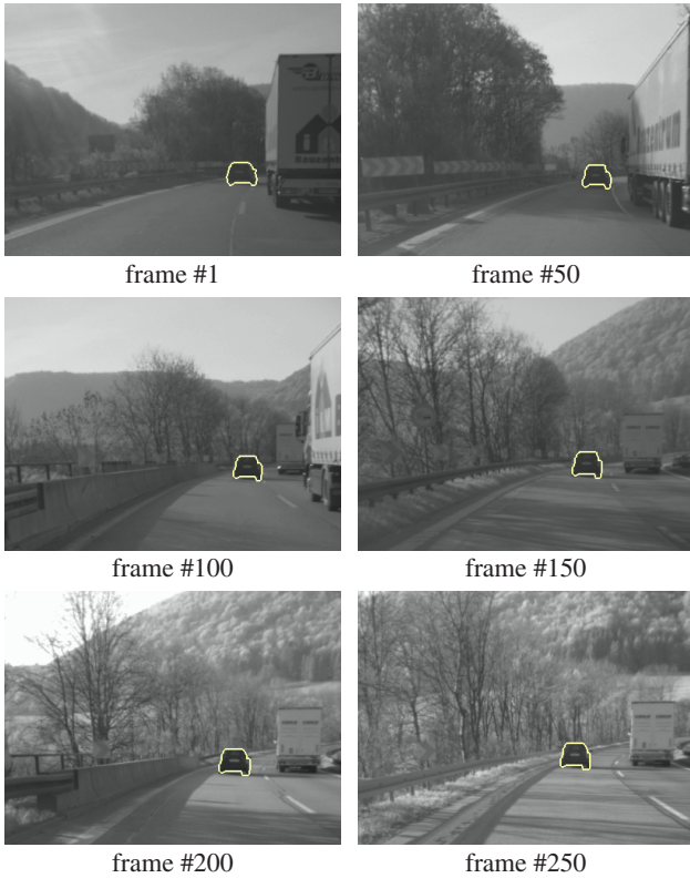
Figure 5. Real-time tracking of a car over 250 frames. Despite sunlight falling directly into the camera and shadow effects, the car is not lost.
