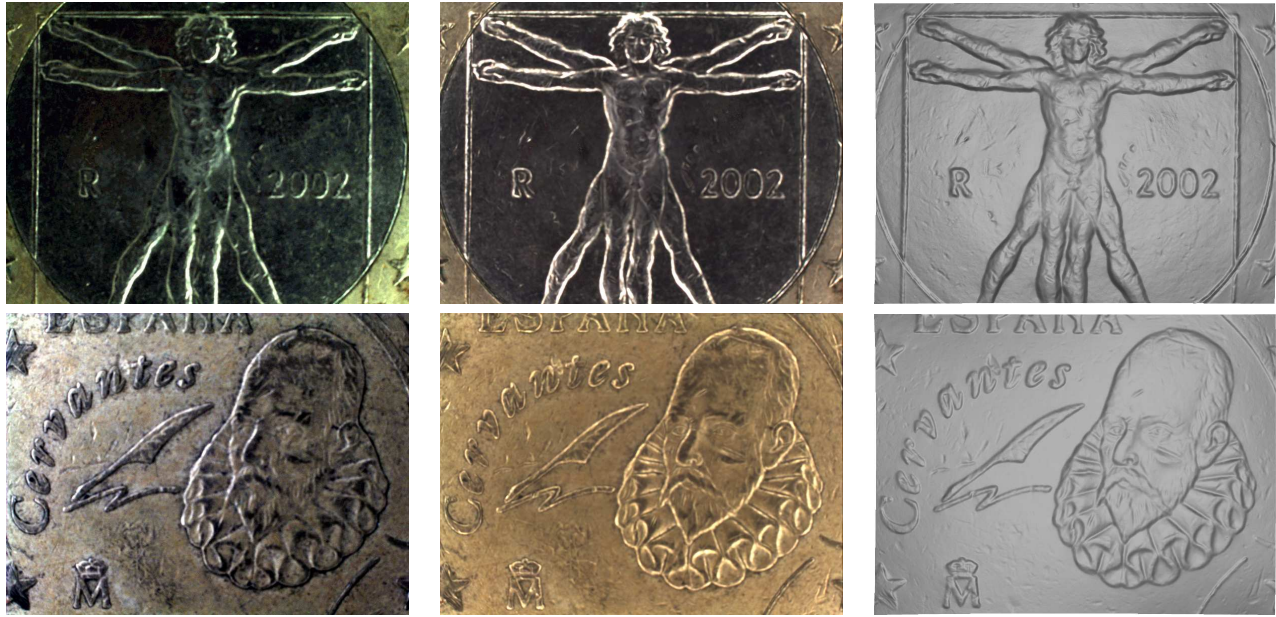
Figure 4. 3D-reconstructions of two metallic coins. From left to right: one of the m = 15 input images, estimated albedo and 3D-reconstruction. First row: Italian 1 euro coin. Second row: Spanish 50 cents coin.
