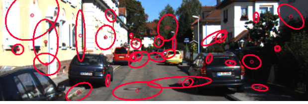
Figure 2. Covariance ellipses for position uncertainties in KITTI seq. 07. The tracks are generated with KLT tracking. Our PNEC correctly considers such anisotropic inhomogeneous error distributions. For visualization purposes only a sub-image with subsampled and enlarged covariance ellipses is shown.
