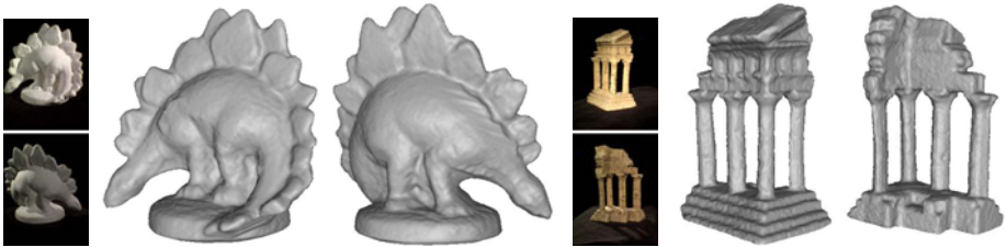
Fig. 5. Middlebury data sets. Two of the input images and two views of the reconstructions obtained with the model in (5) on the well-known “dinoRing” (48 images of resolution 640 \times 480 ) and “templeRing” (47 images of resolution 640 \times 480 ) data sets. See Table 1 for a quantitative evaluation and [22] for a comparison to other approaches.
