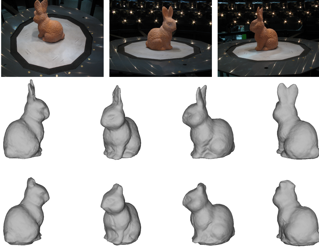
Figure 4. Bunny sequence. First row: Some of the input images (3 of 33) with a resolution of 640 \times 480 . Second row: Reconstruction using the proposed approach. Third row: Reconstruction obtained when the first two terms in (1) are replaced by a ballooning force. Clearly, propagating photoconsistency produces favorable results, while the ballooning force tends to oversmooth the surface.
