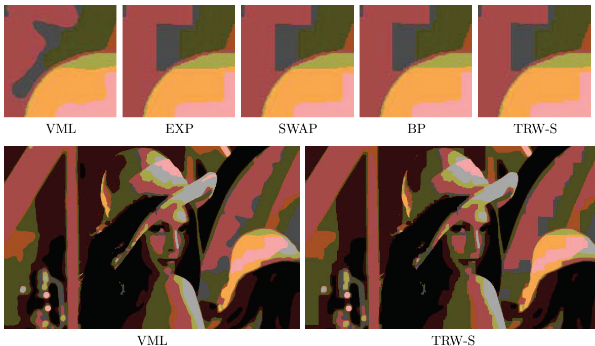
Figure 7. Closeups of 4 \times 4 \times 4 RGB label segmentations (top) using different algorithms reveal a typical problem of discrete approaches: they exhibit a preference for horizontal and vertical region boundaries since they penalize an L^1 -distance instead of the correct Euclidean length [18, 42]. The error can be reduced by increasing the neighborhood connectivity, but only at extremely high costs of memory and computation time. Overall, these metrication errors lead to blocky and visually less pleasing segmentation results (bottom).
