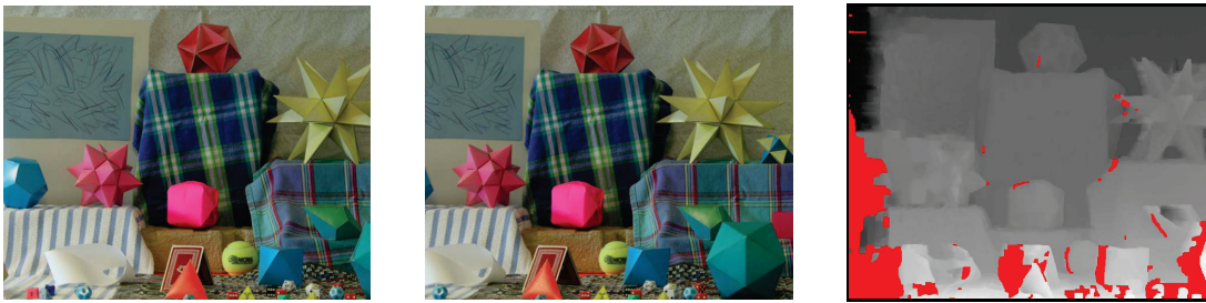
Figure 10. The proposed method can be employed to simultaneously optimize for a displacement and an occlusion map. This problem is also too large to be solved by alternative relaxation methods on current GPUs. From left to right: left and right input images I_L and I_R , and computed disparity and occlusion map; red areas denote occluded pixels. Reprinted with permission from [15, Figure 6], ©2010 by Springer-Verlag, Berlin, Heidelberg.
