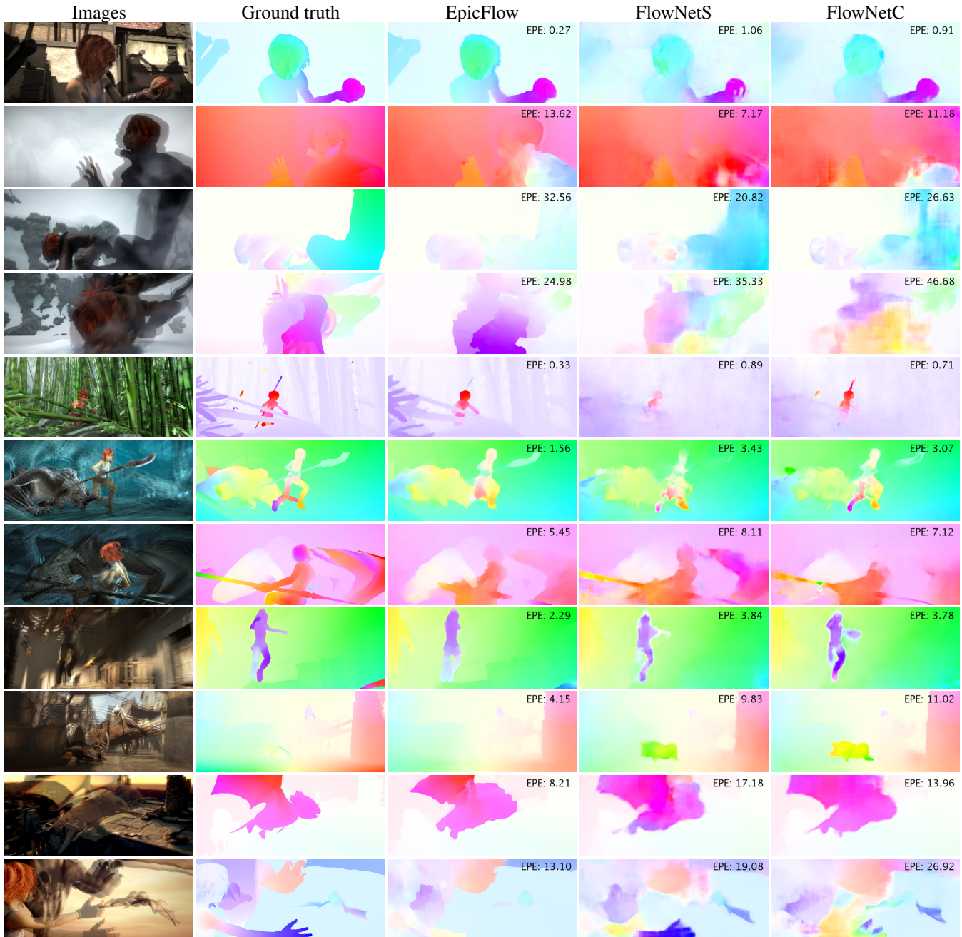
Figure 7. Examples of optical flow prediction on the Sintel dataset. In each row left to right: overlaid image pair, ground truth flow and 3 predictions: EpicFlow, FlowNetS and FlowNetC. Endpoint error is shown for every frame. Note that even though the EPE of FlowNets is usually worse than that of EpicFlow, the networks often better preserve fine details.
