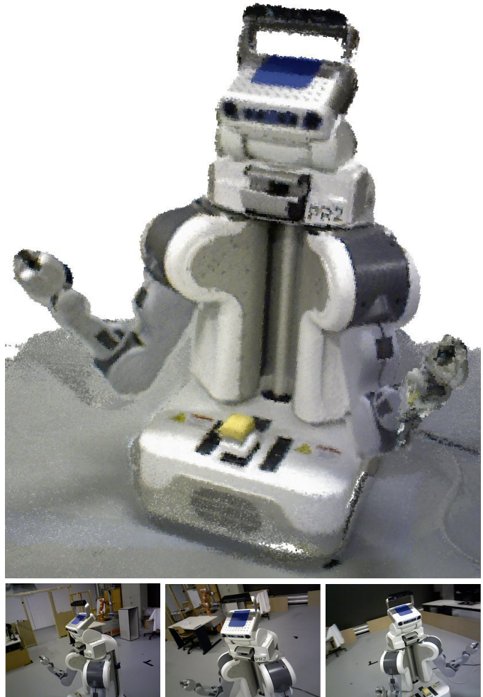
Fig. 1. Top: Occupancy voxel map of the PR2 robot. Voxel resolution is 5 mm. Occupied voxels are represented with color for easier viewing. Bottom row: A sample of the RGB input images.
