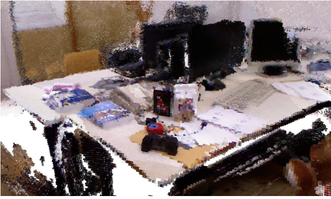
Fig. 6. Occupancy voxel representation of the sequence “fr1/desk” with 1\text{ cm}^3 voxel size. Occupied voxels are represented with color for easier viewing.
