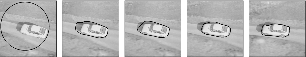
Figure 2: Motion segmentation with an explicit contour for the frames 35–45 from the Avengers sequence. The contour is initialized as shown on the left, then the minimization of (6) is iterated a fixed number of steps on each pair of consecutive frames (the first two images showing frame 35). The comoving shadow is initially associated with the car, but attributed to the background later on. Indeed, due to its semi-transparency, it is unclear whether the shadow is part of the car or not. There is no hypothesis of motion continuity, therefore our approach can also be used for estimating temporally discontinuous motion and for tracking.
