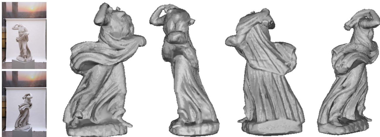
Fig. 11. Reconstruction from the hand-held camera. Two out of 28 input images of resolution 2,048 \times 3,072 and multiple views of the reconstructed surface. Despite severe illumination variations in the input images, the creases of the cloth are recovered in high detail.
