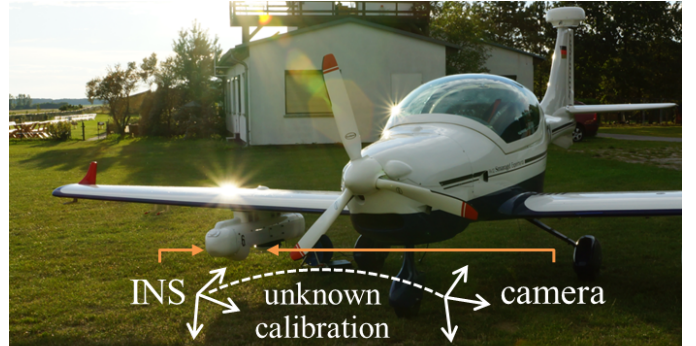
Fig. 1. Our goal is to calibrate the static coordinate system offsets between a camera and an INS, which enables the utilization of the INS measurements as exterior camera orientations. For our flight experiments we integrated the sensors into a payload pod, which was mounted beneath one wing of a manned ultra light airplane.
