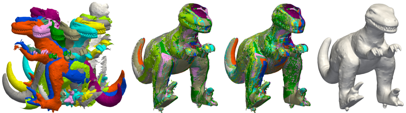
Fig. 16. Fully automatic registration of 12 views of the t-rex model from [2] using the GTR pipeline with Surface Hashes. A set of range images (first column) with unknown initial positions is given; coarse alignment is then performed with our technique and refined with a few steps of ICP (second and third column). The last column shows the final model obtained by Poisson reconstruction [45].
